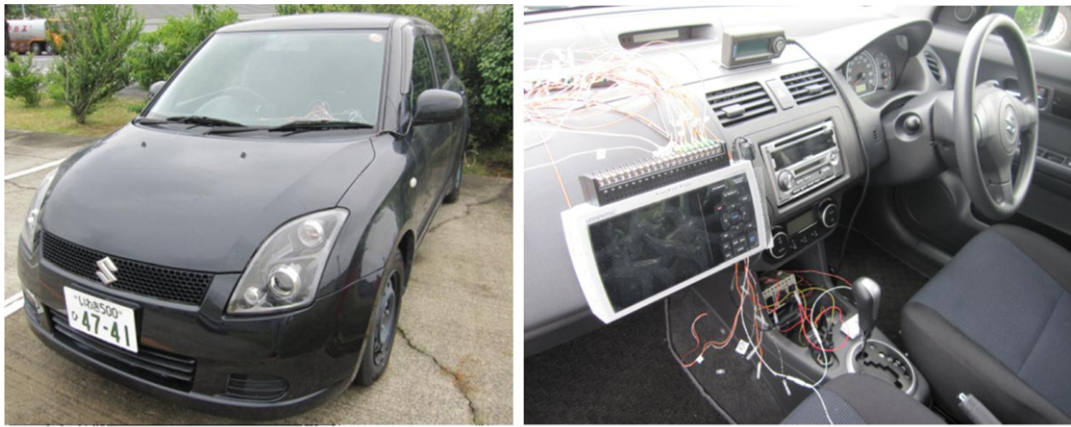
SUZUKI “SWIFT” with Battery Sensor Alternator Control
